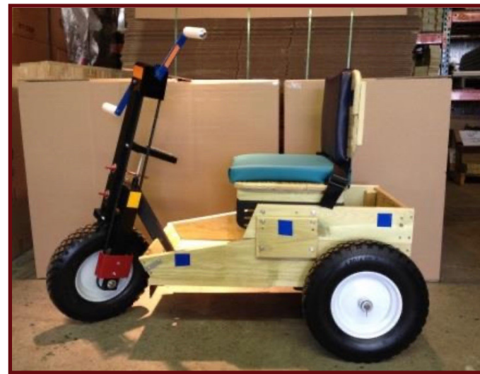
Hand-cranked Personal Energy Transport (PET) carts can go where wheelchairs can't. They can also carry packages.
